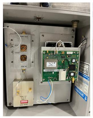
On the right is GPSDO frequency reference with the beacon controller mounted below it. On the bottom left is the carrier synthesizer that produces a signal in the 3460 MHz band that is fed to the tripler on the top right to produce the final 10 GHz signal.
