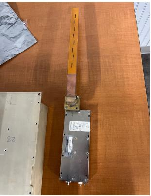
The slotted waveguide antenna is shown mounted on top of the 4.4 W power amplifier. To the left of the amplifier is the heat sink for the amplifier.
