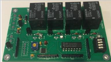
Our Sequencers, SEQ1 and SEQ2, have proven quite popular and we have sold almost all that have been made. But we discovered a small problem with the original design that caused a random time delay when activating or releasing the PTT line. The delay is not very noticeable except when using slow sequence rates. But we felt that this required a new design. The new design uses an interrupt driven microprocessor that instantly responds to changes on the PTT input.
